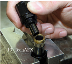
Wet male end of fitting with water
