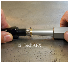
Use awl to 'spread' hose into olive
