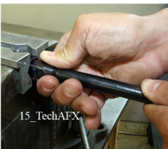
Slide collar to fitting, hand start threads
