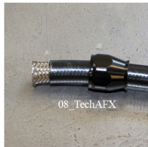
Slide collar on fitting
