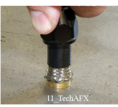
Fully seat olive on end of hose
