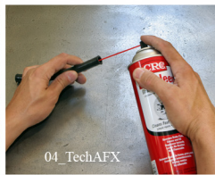
Clean out hose with solvent/air
