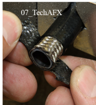
Peel rubber covering off Blackwrap
