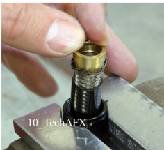
Push 'olive' onto hose end
