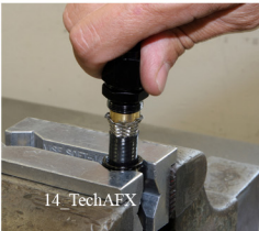
Insert fitting into olive/hose
