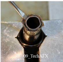
Peel braided steel off conductive core
