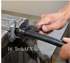
Tighten collar onto fitting
