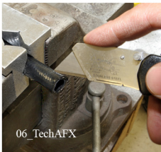
Cut off 7/16 in of sheathing
