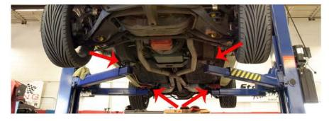
Some vehicles will have a ride-height that is too low to install the Bottom Feed kit without raising it—in these instances, the vehicle will need to be jacked up in the front & placed on two jackstands (locate these at the red arrows). If another type of spoiler is on the vehicle, remove it at this time.
