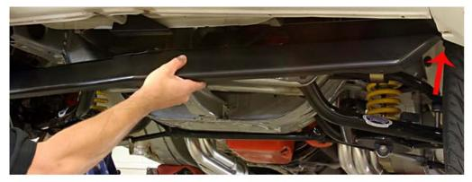
Slide one end of Bottom Feed Air plate over the top of the fender/valence opening (as shown). Make sure the front edge of the main plate is above the rearward lip of the front lower valence panel (this position maximizes the airflow going into the radiator).
