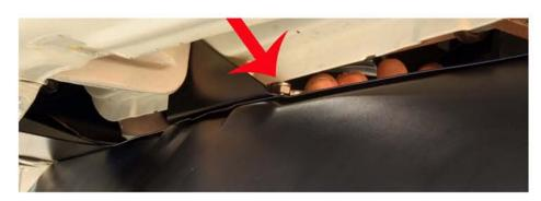
Push the two ¼ inch diameter stainless steel 'L' bracket (with washer on bottom) bolts up through the holes in main plate & 'L' bracket. Hand start the nut (arrow). Tighten with a 5/32 inch Allen and 3/8 inch wrench.
