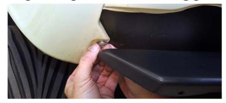
Place the leading edge of the main plate above the rear edge of the front lower valence panel & push spoiler down ½ inch as you position it at body mounting hole. Install the 3/16 inch Allen bolt/washers/nut combo & torque both body mounting bolt assemblies to 104 in-lbs.
