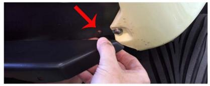
Reinstall bolt/washers/nut assemblies removed in Step 8 by inserting bolt/washer combo downward through each end of mounting plate (arrow) & hand start washer/nylock nut. Use 5/32 inch Allen socket/3/8 inch ratchet with 3/8 inch wrench underneath to tighten bolt/nut combo hand tight.
