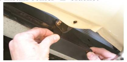
The bracket needs to be lightly pushed forward so the 'L' bracket for the Bottom Feed kit can be slid in between the bracket and core support, as shown. Hand start the factory bolt back in the threaded hole and tighten it to hand tight.
