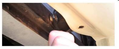
Using the 7/16 inch wrench, remove the center bolt on the lower lip of the radiator core support. This bolt holds a factory bracket that comes off the front lower valence to the radiator core support. This will be reinstalled, so plan on spraying its threads with some WD40 in prep for hand starting it back in the hole.
