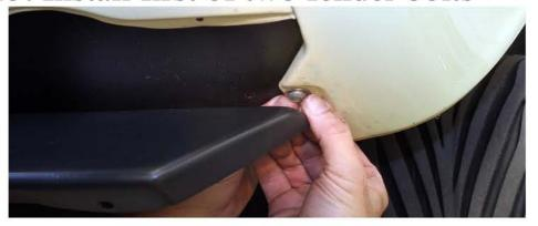
Using provided bolt/washers/nut in plastic bag, insert bolt upward thru fender body mounting hole & Bottom Feed kit mounting plate. Push spoiler slightly forward. Tighten bolt to hand tight with 5/16 inch Allen and hold nut wit 7/16 inch wrench.
