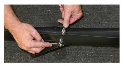
The center 'L' bracket on the main mounting plate for the Bottom Feed kit needs to be removed to install the kit on your vehicle. Using the 5/32 inch Allen socket/6 inch extension/3/8 inch ratchet wrench & 3/8 inch wrench, unthread both bolt/nut
