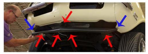
Go back over all of the fasteners and tighten everything to 104 in-lbs. The blue arrows are pointed at the original body fasteners—these will not be accessible now (they should have been torqued to 104 in-lbs in Step 17. Make sure the remaining five fastener combinations are final torqued.
