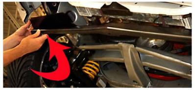
Carefully swing the other end of the Bottom Feed Air spoiler kit rearward in car position about 6 inches as you bring it up the same height as the side you just installed (to maneuver it around the lips of the fender and valence panels).
