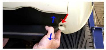
As the body mounting hole for the Bottom Feed Air kit approaches the body mounting flange, push the spoiler and plate apart ½ inch (11). Continue to slide Bottom Feed kit mounting hole towards body mounting hole (1).
