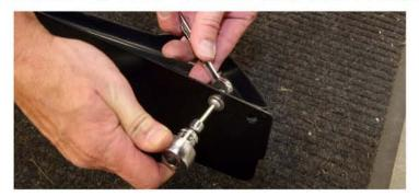
In preparation for installing kit, remove the 5/32 inch fasteners holding the spoiler & mounting plate together at the ends. Use a 5/32 inch Allen with a 3/8 inch wrench underneath. Save these fasteners as they will be reinstalled after the kit is mounted to the vehicle.
